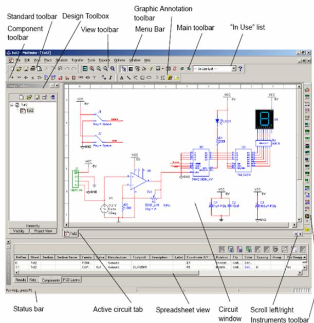
Figure 1. Display of Multisim Environment
