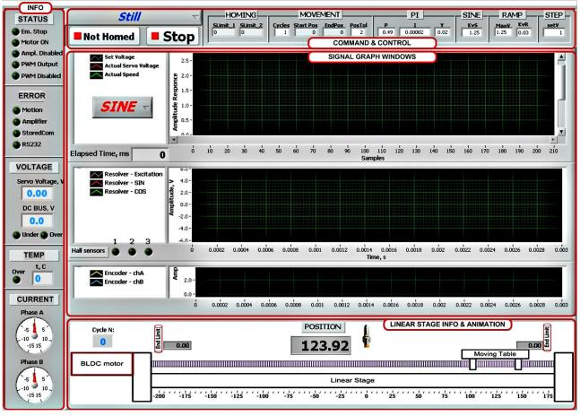
Figure 13. Automation Motion Control Workbench - GUI
