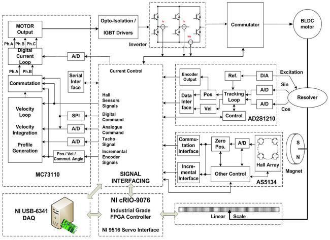
Figure 2. Hardware Structure - Motion Control Workbench
