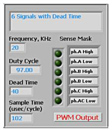
Figure 6. LabVIEW Inverter PWM Diagnostic Window
