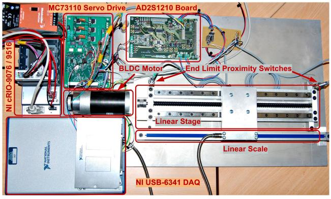
Figure 1. Linear Stage for Motion Control Experimentation
