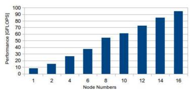
Fig. 5. The HPL (LINPACK) performance of free (t2.micro-based) virtual clusters
