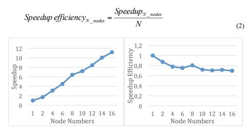
Fig. 6. The speedup and speedup efficiency of HPL (LINPAK) performance of free (t2.microbased) virtual clusters
