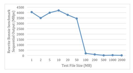
Fig. 3. Bennie rewrite benchmark result. The performance drop indicate the capacity of memory-based disk cache
