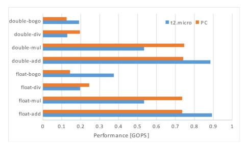
Fig. 2. LMbench results of the performance of t2.micro instance and PC
