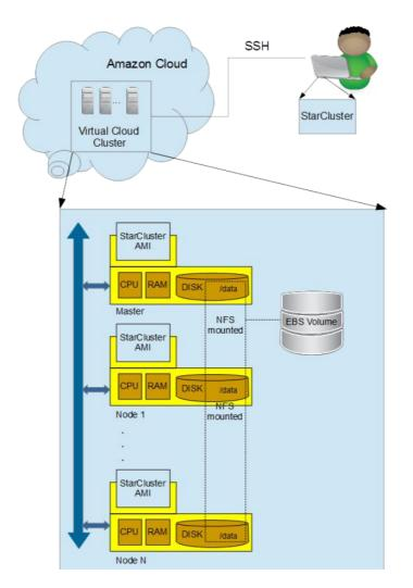
Fig. 1. Architecture of the virtual cluster on Amazon EC2
