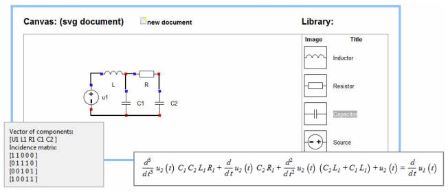
Figure 3. Web application for modeling of RLC circuits
