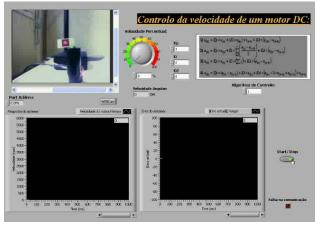
Figure 3. WALC Platform Interface for Control experiments: DC motor control.
