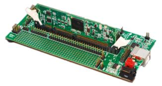
Figure 3. TMS320F28335 Experimenter Kit with controlcard [10]
