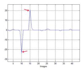
Figure 12. Detection of the blink of an individual by the location of positive and negative sudden change of  $f'(x_t)$ .
