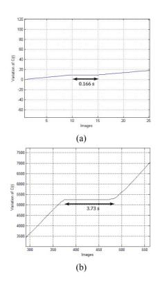
Figure 16. The period of eye closure, (a) the eyes are closed lower than 0.5 s for a normal blinking, (b) the eyes in a state of reduced alertness take a period more than 2 s.
