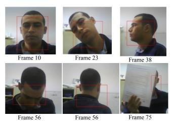
Figure 3. Detection and tracking face results of image sequences using CAMSHIFT algorithm for different conditions
