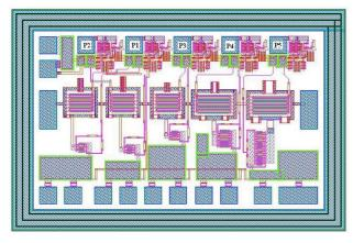
Figure 6. The layout of Wideband 5-bit MMIC digital attenuator with high precision
