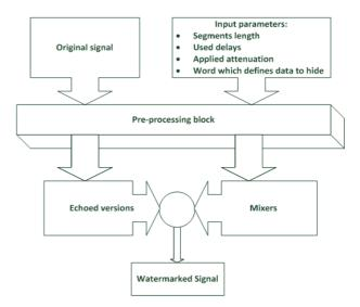
Figure 11. Embedding process scheme
