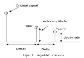
Fig. 2 represents kernels that encode the binary data. These functions are convolved with the original signal in order to create its echoed versions.
