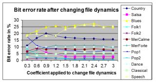
Figure 19. Error rate in watermarks detection after changing dynamics tests
