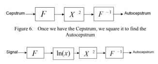
Figure 7. System representation of the autocepstrum
