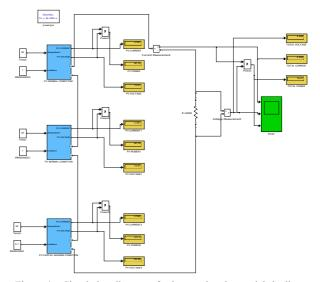
Figure 4. Simulation diagram of solar panel under partial shading conditions
