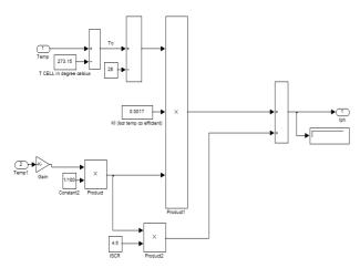
Figure 1. MATLAB modeling of light generated current
