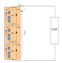
Figure 6. Schematic diagram of PV module with bypass diode
