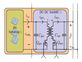
Figure 12. Bidirectional flyback dc-dc converter
