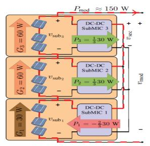
Figure 10. operation of solar panel with subMIC under partial shading conditions
