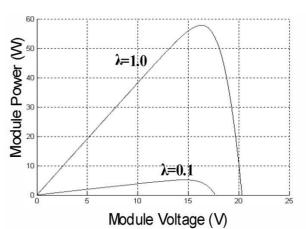
Figure 3. Module power verses module voltage graph
