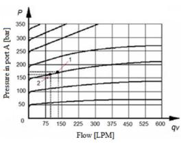
Figure 2. Typical curve of steady state of a relief valve [4]
