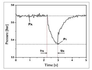
Figure 8. Dynamic behavior of supply pressure using the accumulator with opening of 100% in the VDP.
