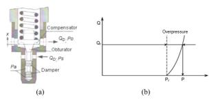
Figure 1. Principle of operation of the pressure relief valve, direct operated. (a) the constructive-way [1] e (b) static feature [10]
