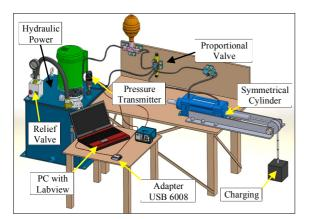
Figure 3. Components of the bench study
