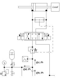
Figure 4. Hydraulic diagram used in the experiment
