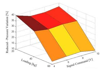
Figure 12. Reduction of variation  $P_s$  from use of the accumulator
