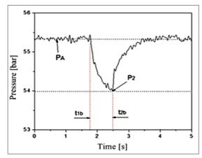
Figure 9. Dynamic behavior of supply pressure using the accumulator with opening of 40% in the VDP.
