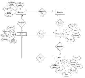
Figure 7. Entity Relationship Diagram in detail for the proposed system
