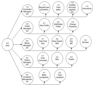
Figure 10. Level 2 DFD for the user logged into the system
