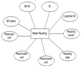
Figure 4. Meter reading attributes for new system
