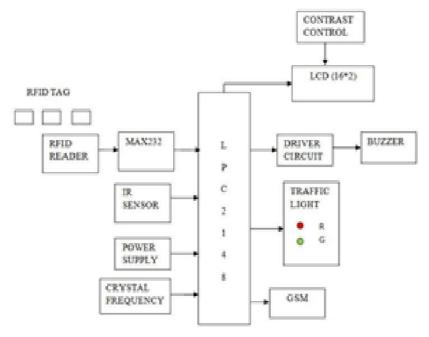
Fig. 2. Block Diagram of Proposed System
