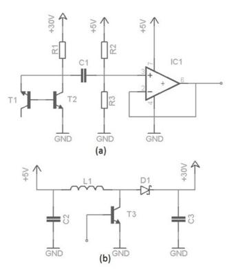
Fig. 8. Noise generator circuit (a) and boost converter (b)
