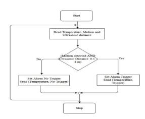
Fig. 6. Sensor node software logic
