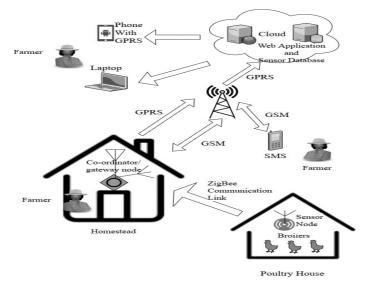
Fig. 2. Poultry Environment Monitoring IoT Model
