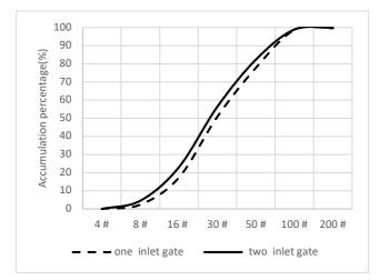
Fig. 9. Comparing Collected particles percentage in hydrocyclone with one and two inlet gates
