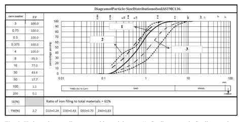
Fig. 6. Hydrocyclone grading curve with one inlet gate (1: Grading curve, 2: Grading envelope according to Building Regulations of Iran [9], 3: Grading envelope according to Iranian Road Construction [10])
