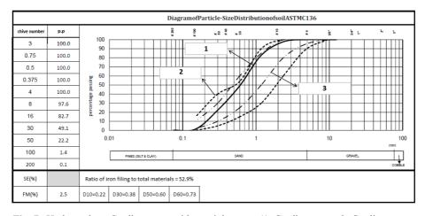
Fig. 7. Hydrocyclone Grading curve with two inlet gates (1: Grading curve, 2: Grading envelope according to Building Regulations of Iran [9], 3: Grading envelope according to Iranian Road Construction [10])
