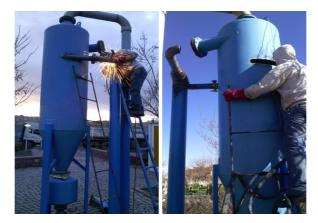
Fig. 4. Stages of cutting inlet gate to hydrocyclone
