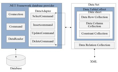
Fig. 2. Structure diagram of ADO.NET
