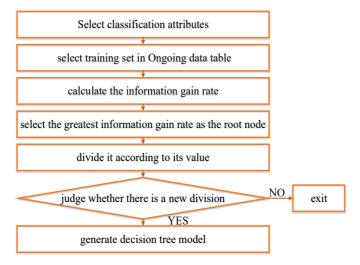
Fig. 3. Iteration process of decision-making tree model building algorithm
