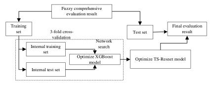
Fig. 7. Flow of model parameter adjustment and update
