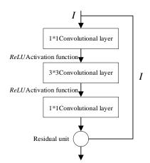
Fig. 5. Residual unit structure
