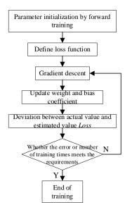
Fig. 6. Flow of the network parameter update algorithm
