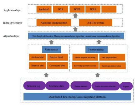
Fig. 6. Architecture of the personalized recommendation system
