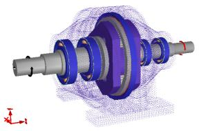
Figure 10. The virtual prototype model of NGW31 planetary gear reducer
