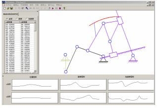
a) Analysis and simulation system of mechanism motion
