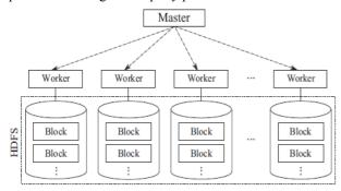
Figure 1. Architecture of Hadoop-based distributed systems
