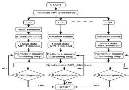
Figure 3. Flowchart for parallel k-means algorithm
