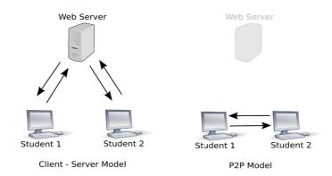
Fig. 1. Communication scheme in a Client-Server model vs communication scheme in a P2P Model.
