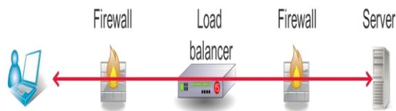
In SLL Offloading mode the handshake is between the browser and the F5 and then invisibly to the User the F5 then handshakes with the target server.
