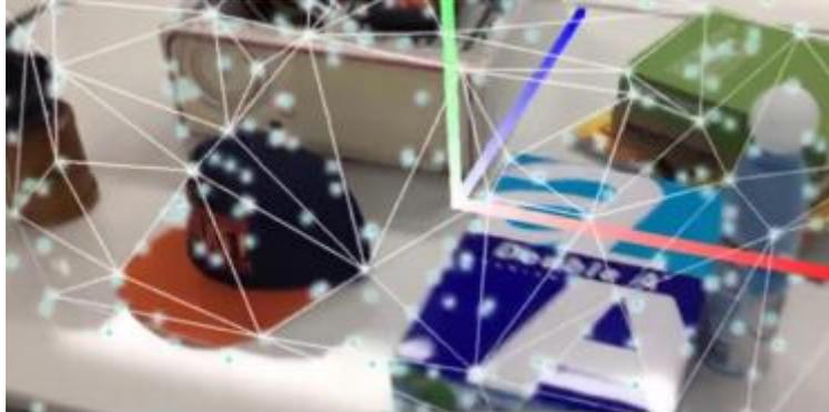
**Fig. 5.** is a feature point display after performing the triangulation, where the goal is to connect a united line to form a triangle that is used as a container for the augmented model.
