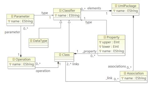
Fig. 2. Simplified UML source meta-model
