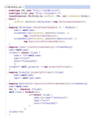
Fig. 7. M2M transformation with QVT From UML to NoSQL model
