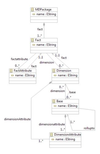
Fig. 4. Simplified Meta-Model of multidimensional schema
