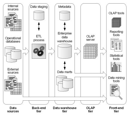
Fig. 2. Typical data warehouse architecture
