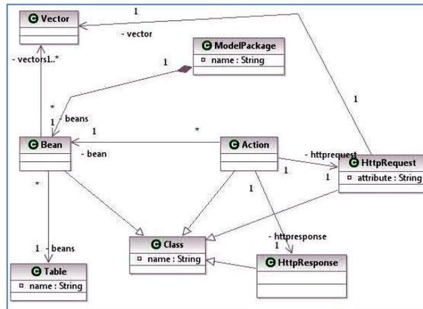
Fig. 4. Simplified Meta-Model of a Model Package
