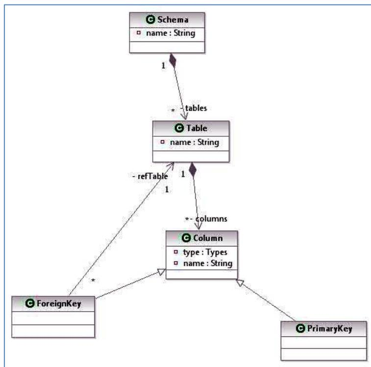
Fig. 3. Simplified Meta-Model of a Relational Database
