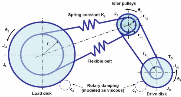
Figure 5. Model of flexible drive dynamics
