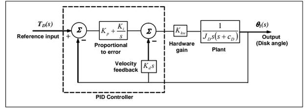
Figure 4. Block diagram for rigid plant PID control
