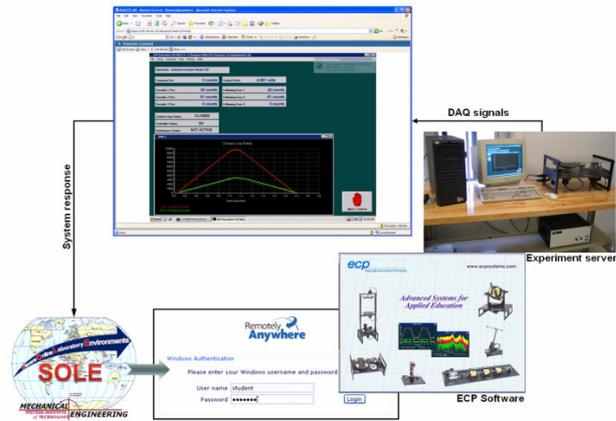
Figure 2. Real-time remote laboratory of emulator system
