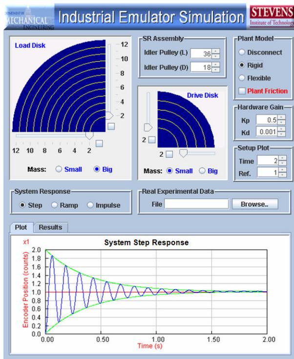
Figure 6. Java applet-based user interface of virtual emulator system
