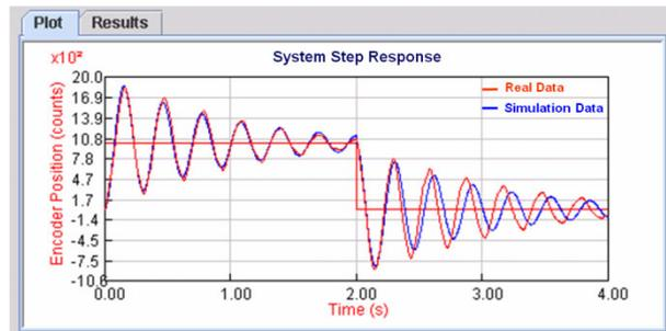
Figure 12. Comparison of real and simulation results (flexible plant)
