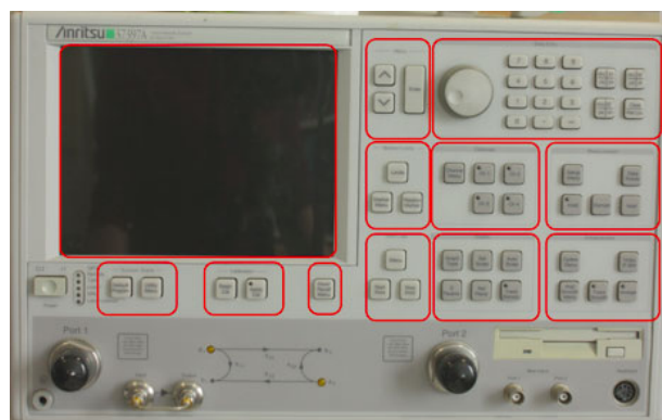
Figure 5. each area can be seen as a widget stored on a Widget server and retrieved by a plug-in within the LMS when the user instantiate a Online Laboratory.
