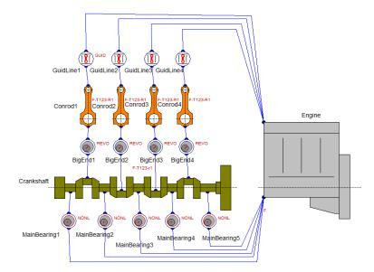
Fig. 2. The diesel engine structural model in the module AVL EXCITE Power Unit
