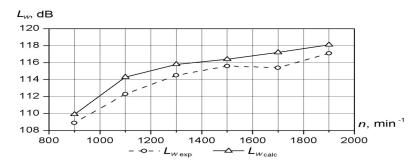
Fig. 7. Experimental and calculated total sound power levels of 8-cylinder diesel engine (D=12 cm, S=13 cm)
