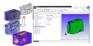
Fig. 3. Preparing the diesel engine calculation model in the module AVL EXCITE Acoustics
