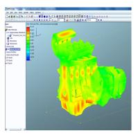
Fig. 5. Example of the results of calculating the speed of vibrations of the external surface of the engine in module AVL EXCITE
