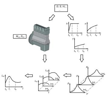
Fig. 6. The sequence of the engine structure-borne noise calculation for the transient mode
