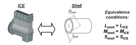
Fig. 1. The model of the equivalent cylindrical shell for the engine noise calculation
