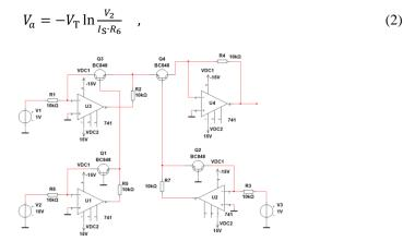
Fig. 6. Simulation circuit of the single-quadrant multiplier in MultisimTM [9]
