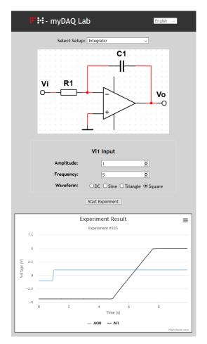
Fig. 10.Web client with experiment result
