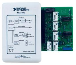
Fig. 4. Final lab PCB connected to a NI myDAQ. The experiment is again the single-quadrant multiplier
