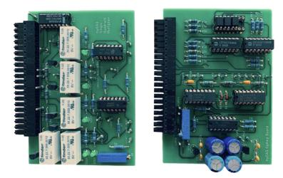
Fig. 5. Single-Quadrant Multiplier Board (left) and Operational Amplifier Board (right)
