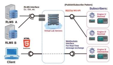
web client can either directly connect to a Virtual Lab Server instance provided by the Dispatcher, or connect via one of the aforementioned RLMS systems.
