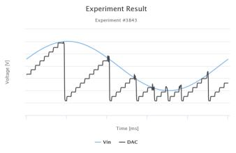
Fig. 8. Example of an experiment result (Ramp ADC)
