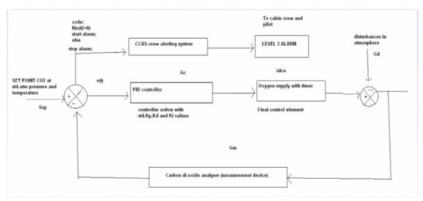
Figure 1. Feedback action used in ALSD in airplanes
