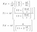
Here t=time constant; td=dead time; Ti=Integral time; Td=derivative time;
