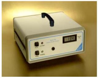
Figure 4. The Model 906 can have the sensor located remotely up to a distance of 2-3 feet from the unit.
