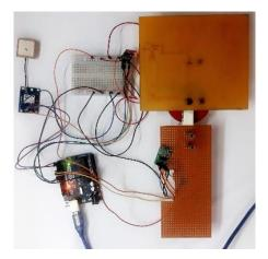
Fig. 3. Circuit implementation of complete system
