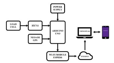
Fig. 2. Hardware block diagram of Easy-Weigh-Out system
