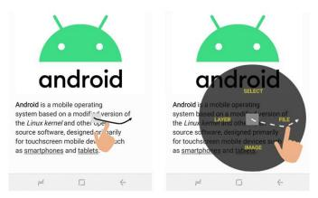
**Fig. 2.** Enhancing the visibility of underlying application content by utilizing semi-transparent floating pie-menu widget (instead of typical full-screen linear-based menu)
