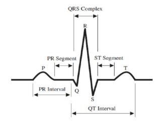
Fig. 1. ECG signal PQRST Components
