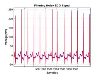
Fig. 5. Noise Filtered ECG Signal
