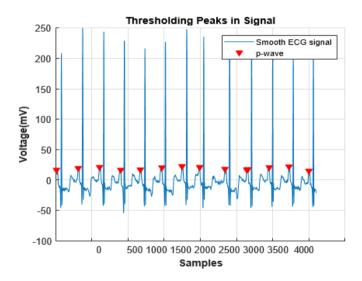
Fig. 8. P wave peak detected in ECG signal
