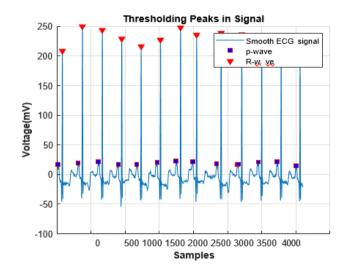
Fig. 6. Thresholding of Peaks in ECG Signal
