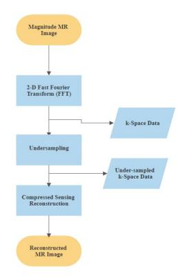
Fig. 5. Flow Diagram for the reconstruction of MR image using magnitude signal
