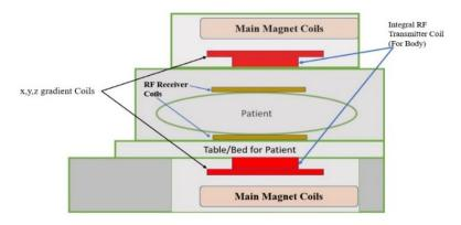
Fig. 1. Diagram representing the relative position of RF receiver coil, RF transmitter Body coil and x, y, z position of the gradient coil
