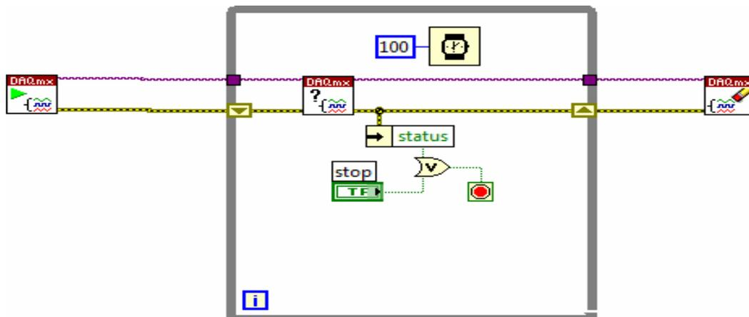
Figure 1. Low Level DAQmx Code for Clock Signal Generation in LabVIEW
