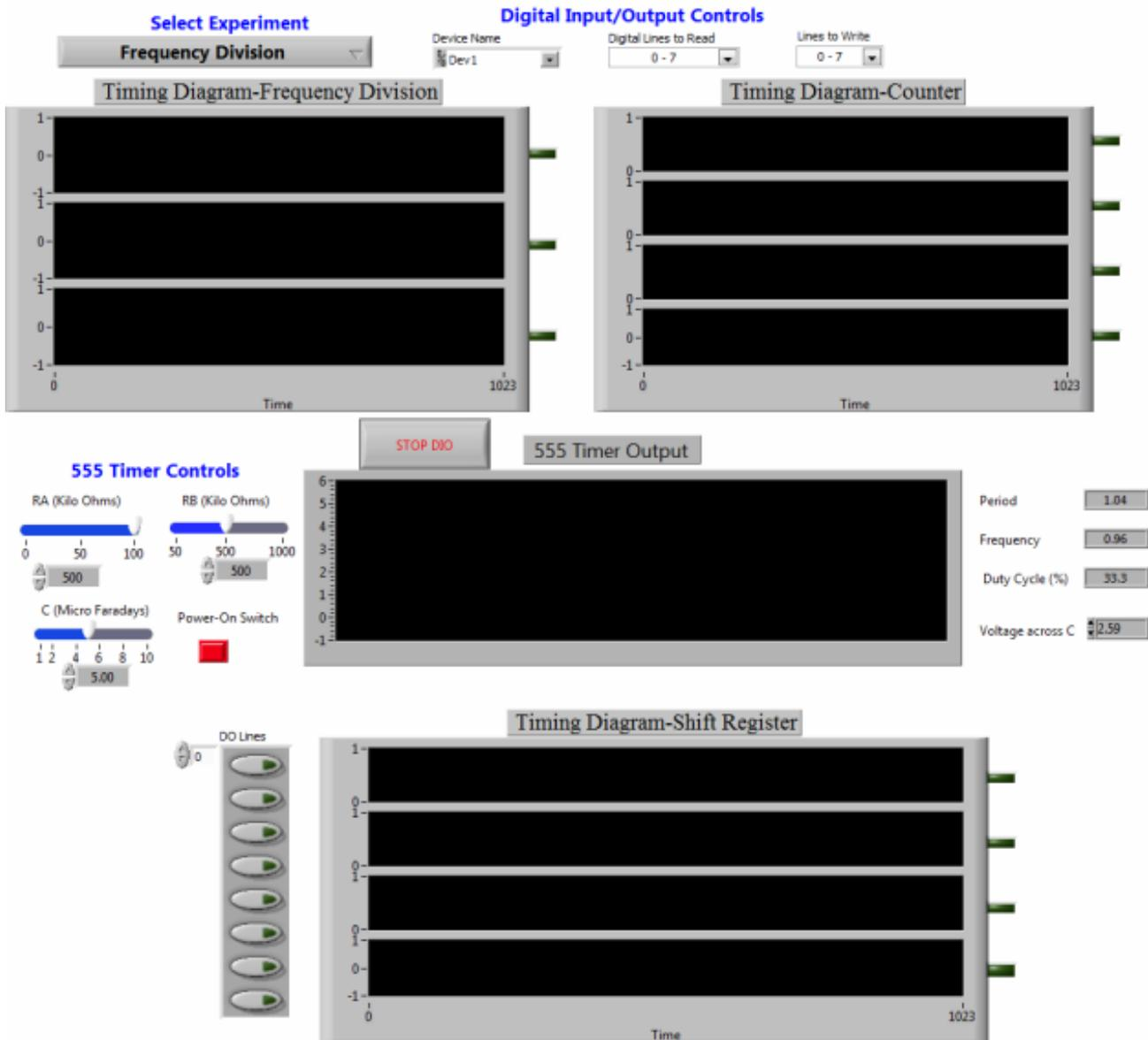
Figure 5. Sequential Logic User Interface
