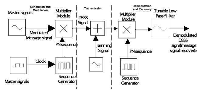
Figure 3. DSSS Block Diagram
