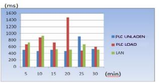
loaded PLC technology was outstanding in 4 of the 6 samples. This even further proves the efficacy of the technology in industrial environments and confirms the success of the results which could be seen using the proto-type, where at no time did some activation fail to take place.
