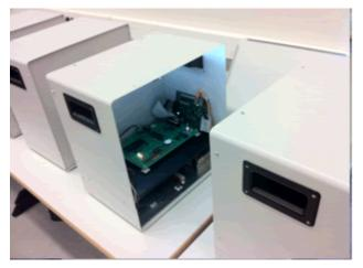
Figure 4. WebLab Deusto PIC into a WebLab Deusto Box.
