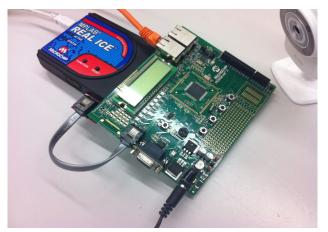
Figure 7. PICDEMNET2 Board used in E-PRAGMATIC course.
