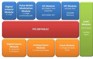
Figure 6. WebLab Deusto PIC Modular Structure.
