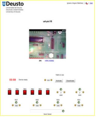
Figure 5. WebLab Deusto PIC Interface.
