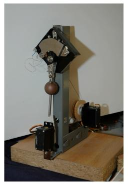
Figure 2. Experimental apparatus of the Pendulum Experiment to be deployed on e-lab.
