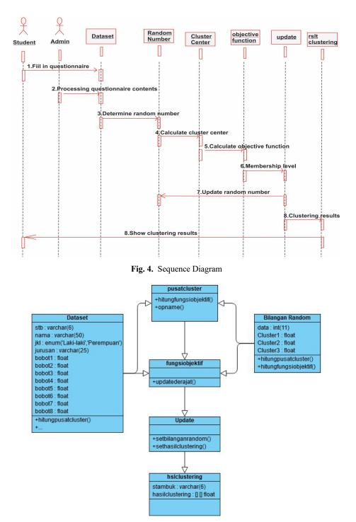
Fig. 5. Class Diagram Application
