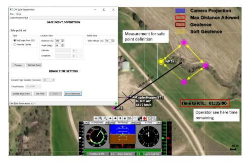
Fig. 9. Software interface for safe parameters Configuration.
