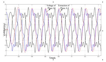
Figure 5. Fundamental positive sequence voltage extraction result of phase A under unbalanced and distorted voltages
