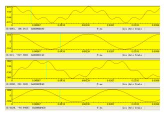
Figure 10. The waveform of input voltage and extracted fundamental positive sequence voltage when the system has achieved stability (from top to bottom respectively are phase A voltage waveform, extracted voltage of phase A, phase B voltage waveform and extracted voltage of phase B)
