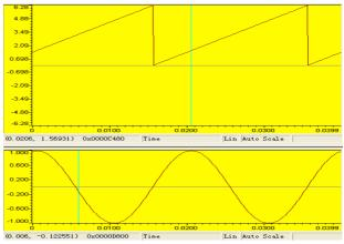
Figure 11. The waveform of SPLL output and its corresponding sine value when the system has achieved stability
