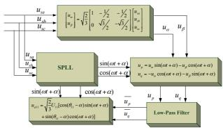
Figure 1. The principle block diagram of fundamental positive sequence voltage detector
