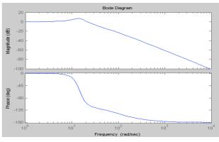
Figure 4. SPLL bode diagram (above is for magnitude, below is for phase)
