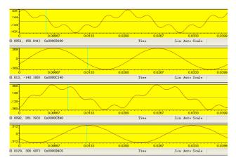
Figure 8. The waveform of input voltage and extracted fundamental positive sequence voltage at the first few cycles (from top to bottom respectively are phase A voltage waveform, extracted voltage of phase A, phase B voltage waveform and extracted voltage of phase B)
