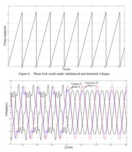
Figure 7. Fundamental positive sequence voltage extraction result of phase A when the harmonic and negative components disappear
