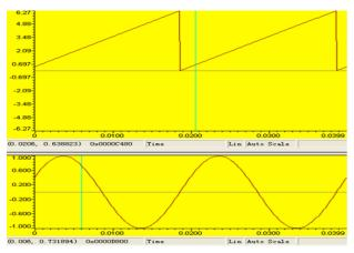
Figure 9. The waveform of SPLL output and its corresponding sine value during the first few cycles
