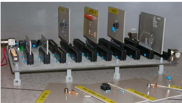
Figure 2: The motherboard and the circuit cards
