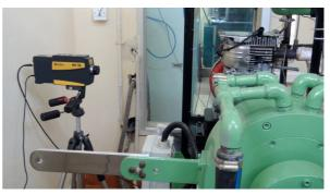
Figure 3. Laser vibrometer for engine vibration measurements
