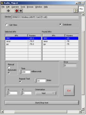
Fig. 6. Data acquisition and radio map building panel
