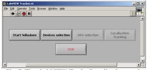
Fig. 7. The "LabVIEW Tracker" application panel. The application starts when the "Localisation – Tracking" command is selected
