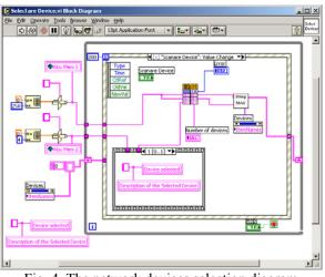
Fig. 4. The network devices selection diagram
