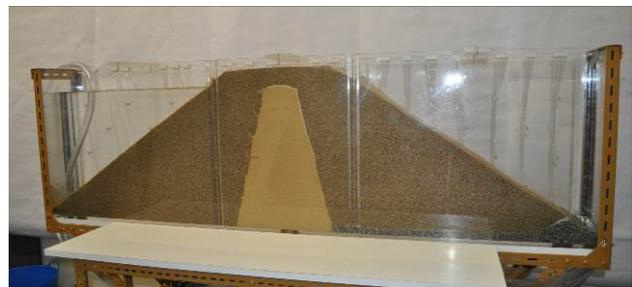
Figure 5. Small scale model of earth dam with central core, drainage blanket and toe drain.
