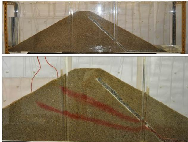
Figure 1. Small scale earth dam with a chimney drain (top); flow lines obtained with injection of color fluid (bottom).
