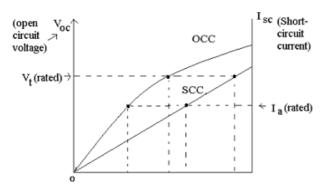
Figure 12. OCC & SCC characteristics
