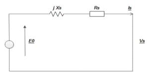
Figure 10. Circuit diagram to perform short circuit characteristic (SCC)
