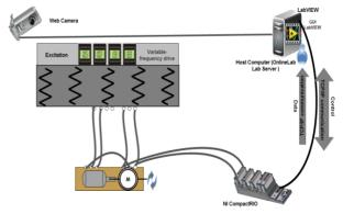
Figure 6. The Architecture of the OnlineLab laboratory
