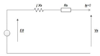
Figure 9. Circuit diagram to performopen-circuit characteristic (OCC)
