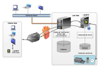
Figure 3. The architecture of the ISA OnlineLab laboratory
